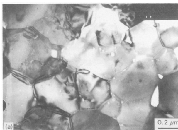
Figure 2 Microstructure of 0.1 mol % Y_2O_3 doped alumina, (a) after heat treatment for 72 h at 1650 °C in air, (b-c) after heat treatment for 24 h at 1350 °C in air.
